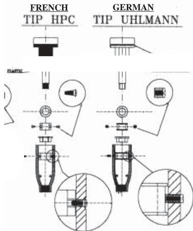
There are two designs in foil points, each with a weakness. The German design has a nice steel sleeve to protect the tip insulator, but leaves the screw heads unprotected. The screws are easily damaged, making servicing of the tip impossible.
